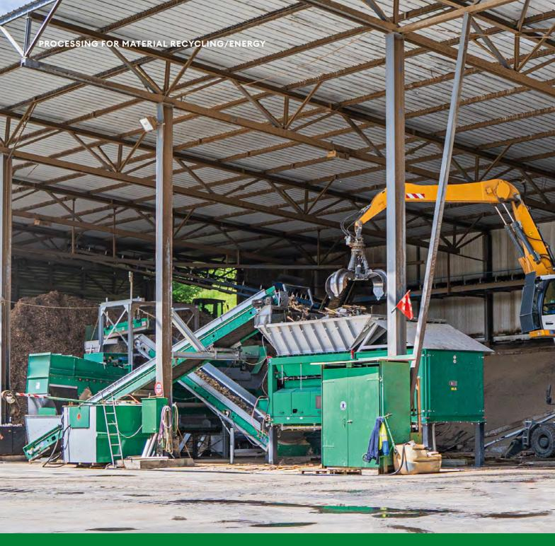
Depending on requirements, a Multistar star screen is used to generate two or three fractions. The overlengths from screening are fed back into the shredder by conveyor. The desired particle size can be obtained simply by adjusting the rotational speed of the star shafts.
