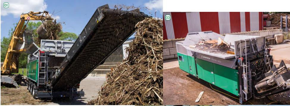
Green waste, woody biomass A high throughput of bulky vegetation is made possible by the generously dimensioned feed area, folding hopper and counter-rotating teeth. Blockages from wet material and high grass content are practically impossible. The teeth clear the screen baskets on every revolution.
